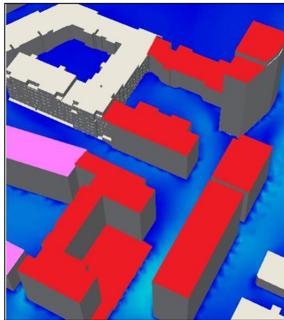
Figure 13.61: Flow Velocity Results at Z=1.5m Above the Ground - Direction: 136°. - Direction: 136°.
