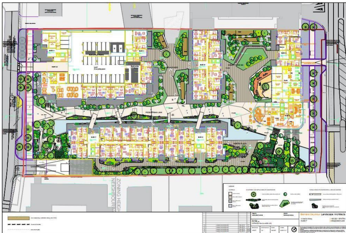
Figure 13.52: Ground Level Landscaping Design Implemented in the Critical Areas Detected by the Preliminary Wind Analysis.
